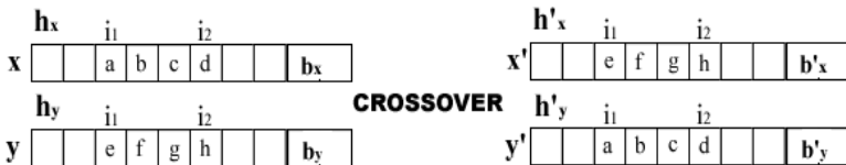
Fig. 3. An example of crossover on the head
